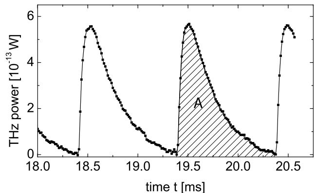
**Fig. 3** TES signal showing resolved THz pulses obtained at 0.76  $\text{mJ}/\text{cm}^2$  laser pulse fluence; area A corresponds to pulse energy of 0.21 fJ
