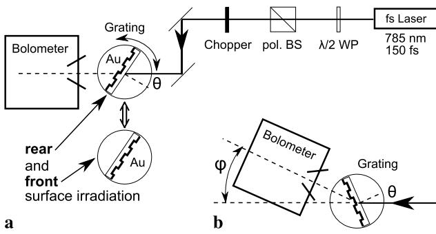
**Fig. 1** (a) Scheme of experimental setup for generation and detection of THz radiation: fs laser,  $\lambda/2$  wave plate (WP), polarizing beam splitter (BS), chopper, nanograting, and bolometer (b) modified setup for measuring the angular distribution of the THz radiation
