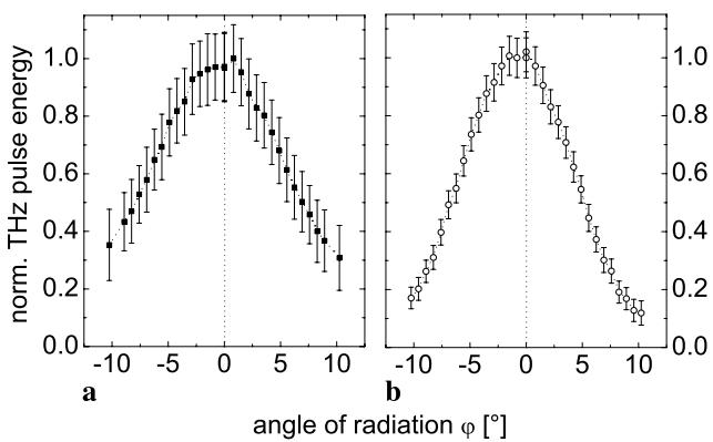
**Fig. 5** Normalized THz pulse energy as a function of the emission angle  $\varphi$  obtained with a grating of 320 nm bar width for both laser irradiation configurations: (a) rear surface at  $\theta_r = (10 \pm 1)^\circ$  (b) front surface at  $\theta_f = (8 \pm 1)^\circ$ ;  $\varphi = 0^\circ$  is the direction of the laser beam (Fig. 1b)
