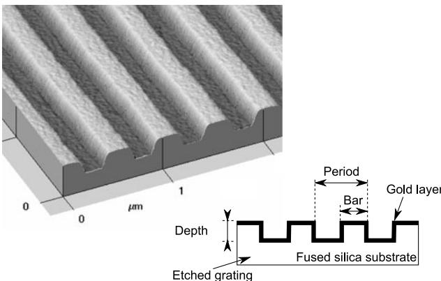
**Fig. 2** AFM picture of a gold coated nanograting in fused silica with 500 nm period, 90 nm depth, 250 nm bar width, and 30 nm coating thickness
