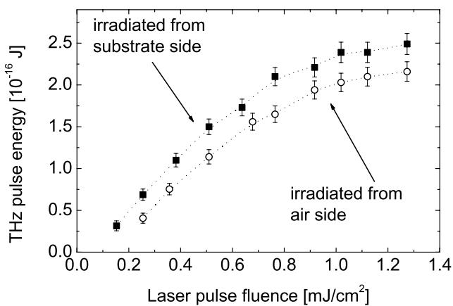
**Fig. 4** THz pulse energy as a function of incident laser pulse fluence for both configurations: irradiation of rear (■) and front surface (○)
